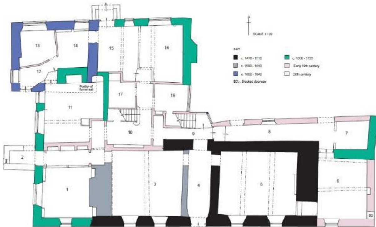
Fig ??: East Worlington House, ground floor plan showing developmental phasing
