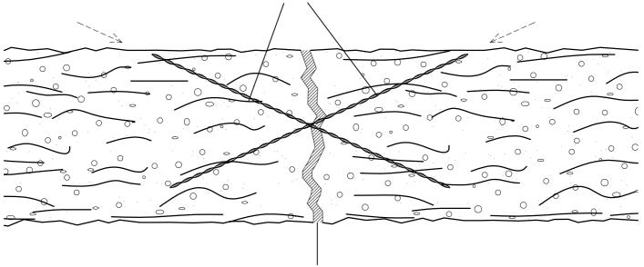
Crack to be raked out and filled with lime putty or hydraulic lime mortar. If cracks exceed 25mm width fill with pieces of broken brick or clay tile in lime mortar.
